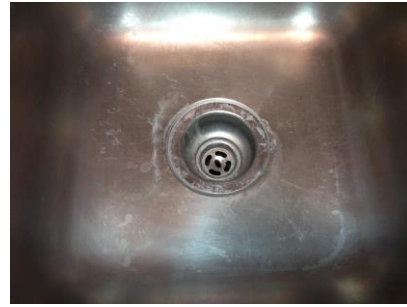
Water Stains on Stainless Steel
